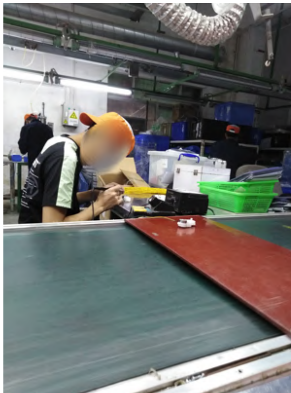
(Soldering position without an exhaust fan)
