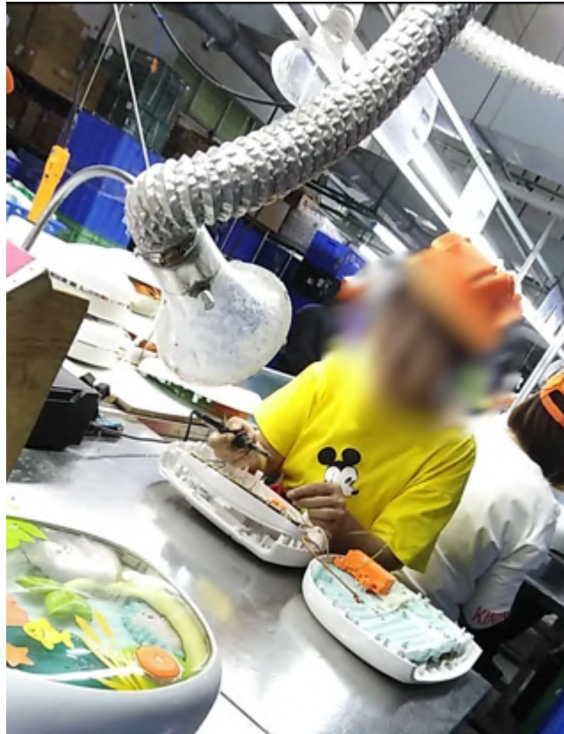
(Soldering position with exhaust fan)
