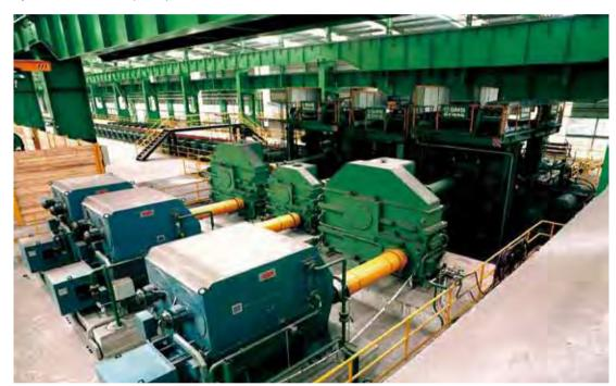
Electric motors (in the foreground) driving a metals rolling mill
